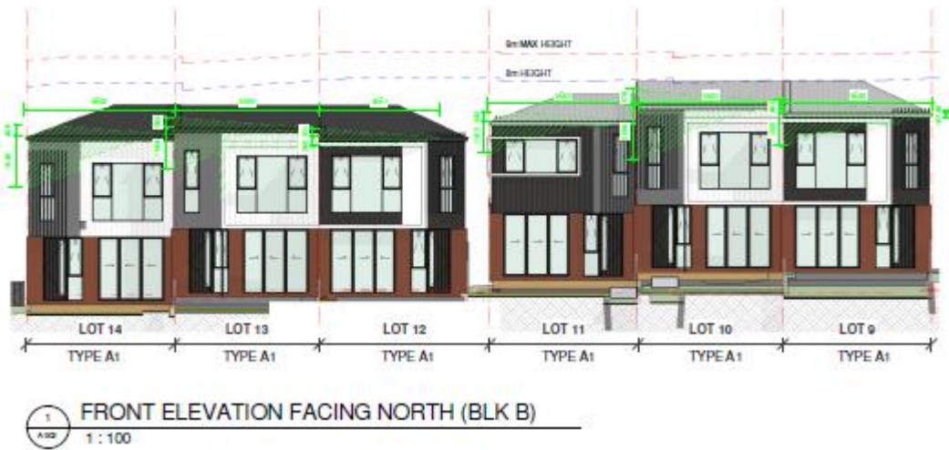
Figure 17: Partial front (northern) elevation of Block B
